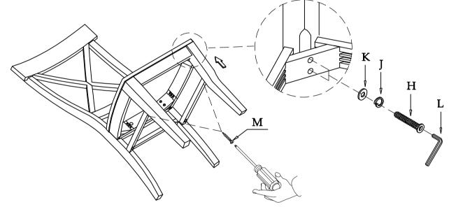
Step 5: Using a Phillips head screw driver to tighten all screw
